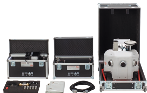
From left to right: Optional wheel sensor, battery with power cable and rain cover, sensor system.
